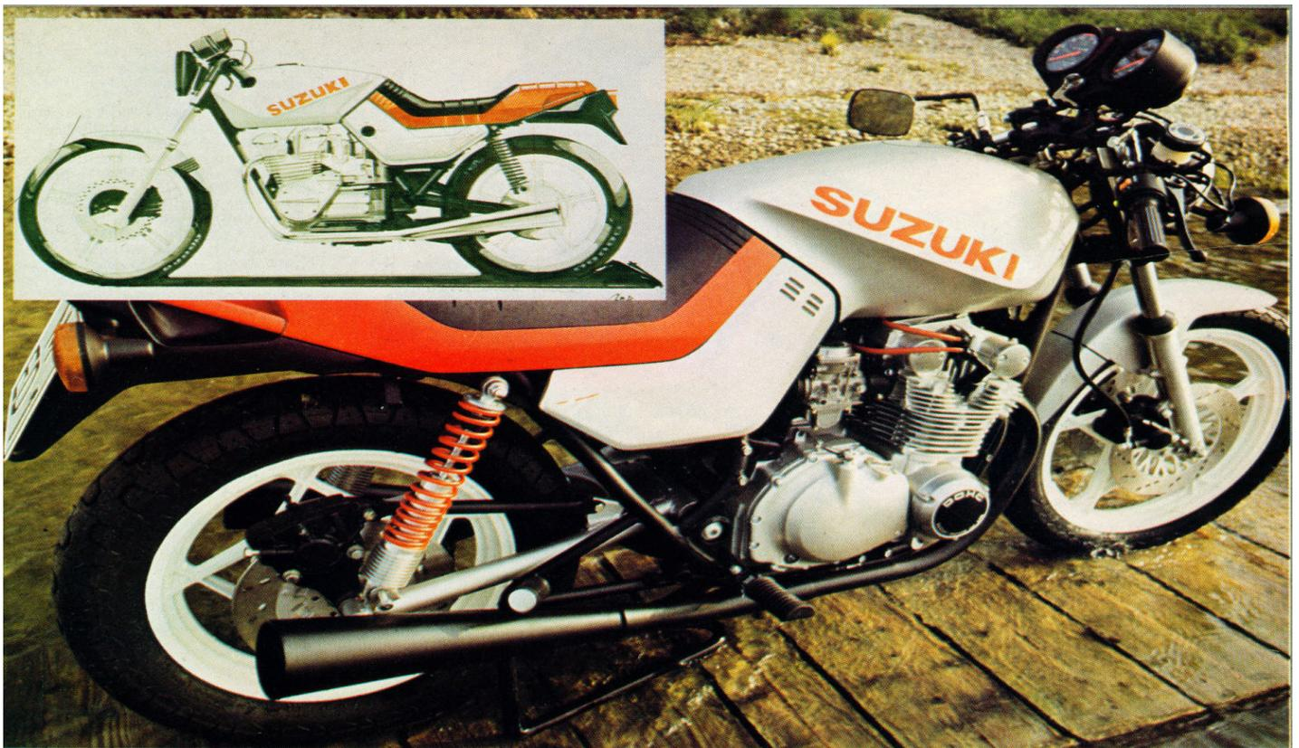
Rare picture of prototype, note lack of rear brakes, normal GS range clocks, no stands, lack of orange brakes, pre 1981 indicators, fairing bracketery, and wild drop bars. The seat also incorporated a grab rail.
