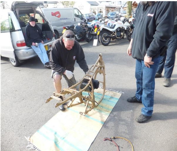
So it begins, Airbox first..... lay the engine on its side, put the frame over it.
