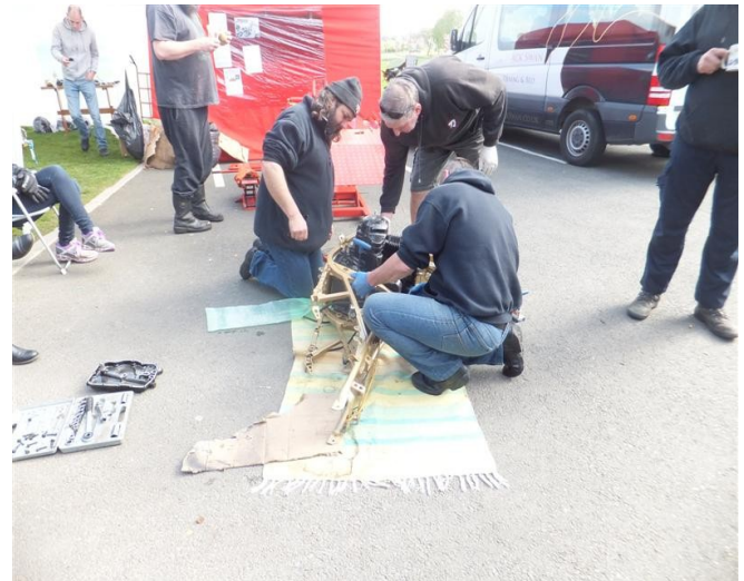
So it begins, Airbox first..... lay the engine on its side, put the frame over it.
